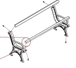
Place the rung between both castings. Attach the rung with bolt configuration (parts D and E) as shown.
