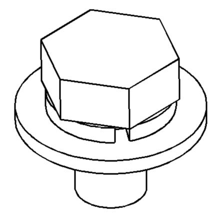
Lock washer when TOOL tightened DO NOT OVER TIGHTEN
