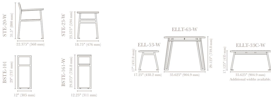
See product specifications for further details. Drawings are not to scale. Our TGIC powder-coating averages 8-10 mils (200-250 microns) thick and is applied in-house to ensure the highest level of quality. Offered in 12 standard and metallic colors, new matte finishes, plus a full range of RAL colors with available color matching. Additional cost may apply.
