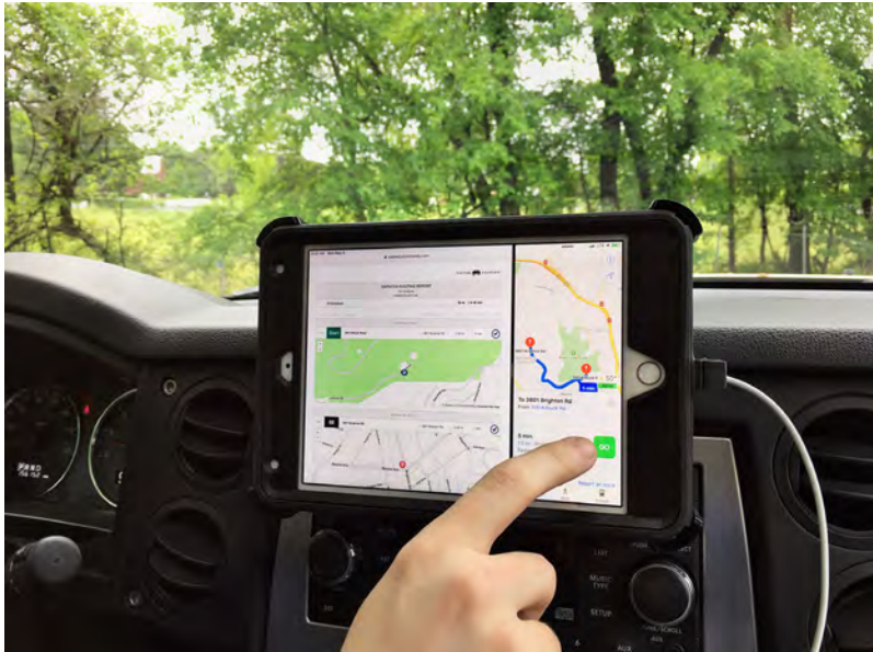
The Relay routing system navigates to only the containers in need of collection
