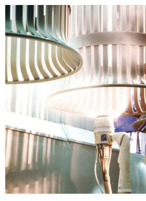
in succession, the company calls it a continuous batch system. In addition to saving energy, continuous batching promised to simplify powder application: The conveyor could halt loads of parts in the powder enclosure and give the applicators more time with the parts. This would allow the applicators to inspect the coating thoroughly before the parts entered the cure oven, which would reduce rework. The next concern was how to apply powder to the hot surfaces.
